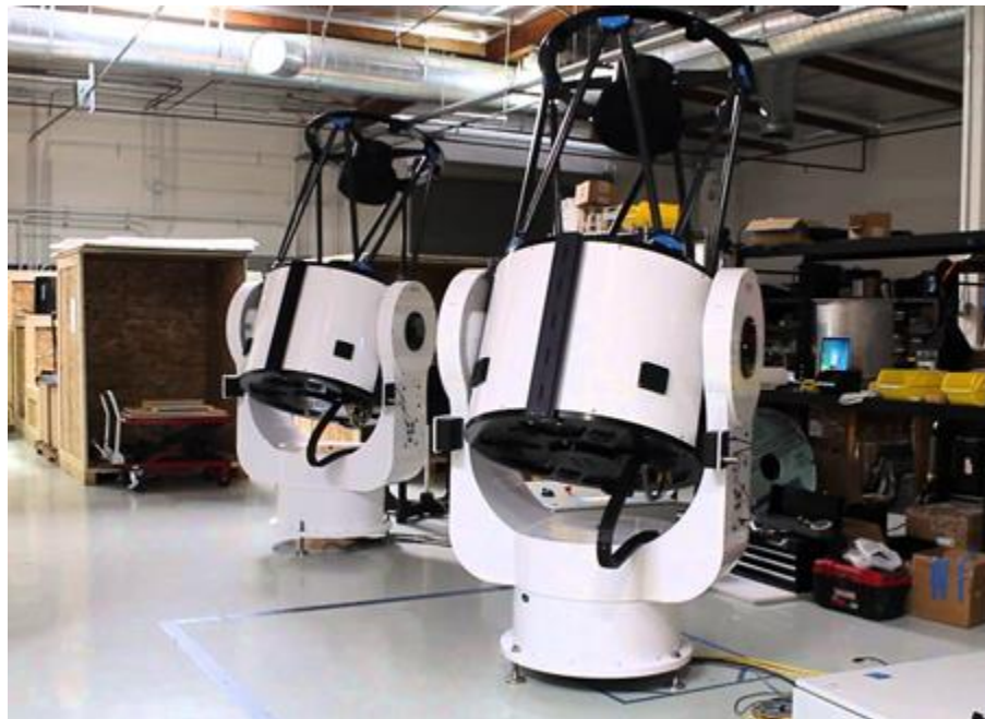
Figure 2: The PlaneWave Instruments CDK-700 0.7-meter fully robotic telescope at Great Basin Observatory. This direct-drive, production telescope features dual Nasmyth ports and is an example of reverse innovation.
