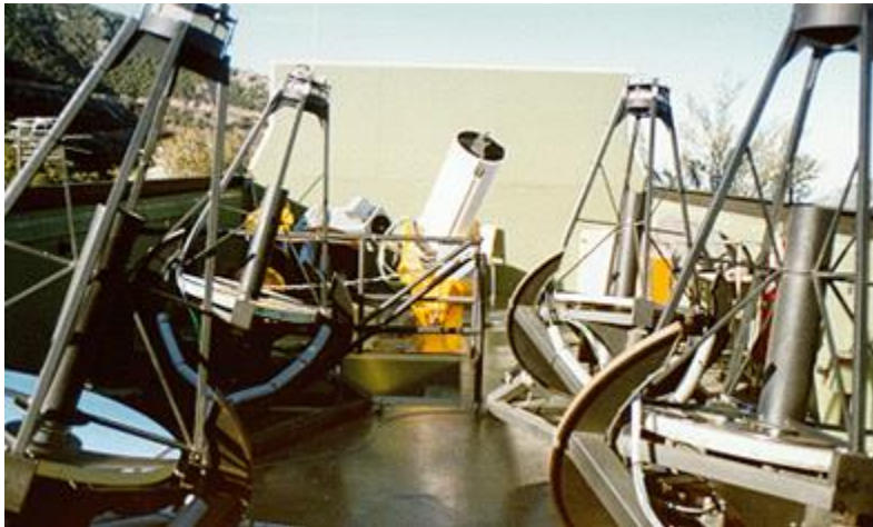
Figure 1: Seven fully robotic telescopes at the totally automated Fairborn Observatory on Mt. Hopkins in the late 1980s. Remote access was via 9600 baud modems over the telephone lines. These seven telescopes specialized in high precision, time-series photometry. The first exoplanet transit was observed with one of the four 0.8-meter telescopes in 1999.
