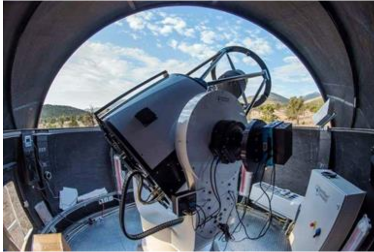
Figure 2: The PlaneWave Instruments CDK-700 0.7-meter fully robotic telescope at Great Basin Observatory. This direct-drive, production telescope features dual Nasmyth ports and is an example of reverse innovation.
